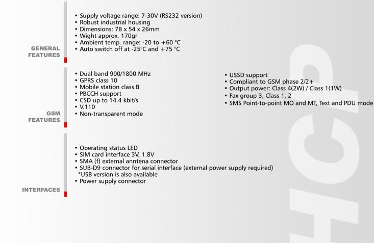
\* USB version of the HCP hit 39 is powered by standard USB interface and does not require external power supply.
