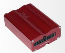
HCP Roadstar is tracking terminal based on GPS/GPRS technology. It can be adapted to almost any kind of end-user needs because of his Java<sup>™</sup> programmable ability.
