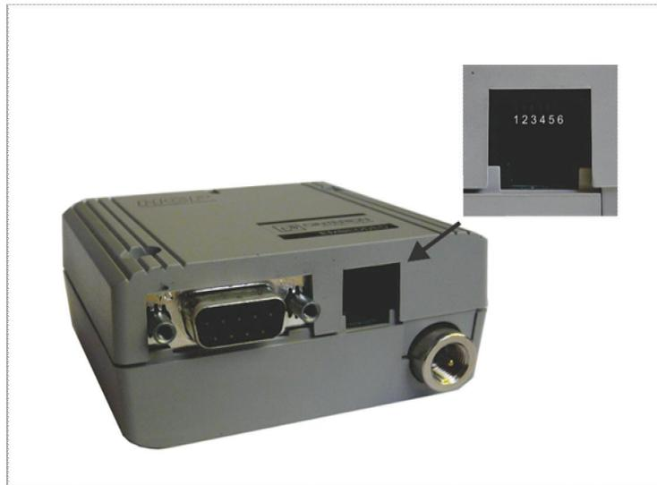
**Figure 3.** Power supply connector
