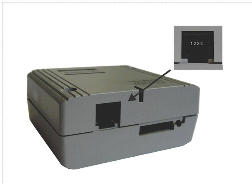
**Figure 5.** Audio interface connector
